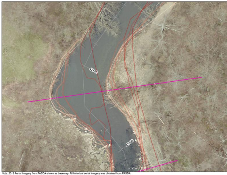
Figure 2: Aerial photograph analysis showing bank retreat along an outer meander bend within the study reach. The dark lines indicate the location of the stream banks in 1996, while the lightest lines indicate the position of the banks in 2020.
